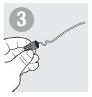
Attach wire nuts to end of each conductor wire.
