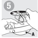
Cover with blank-up canopy (A). Make sure all wires are carefully placed inside of box and blank-up.
